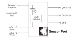
Note: The power output from Unswitched and Switched are both metering.
